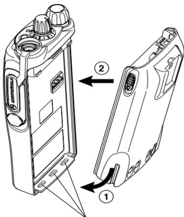
1. Fit the extensions at the bottom of the battery into the slots at the bottom of the radio's body.
