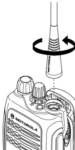
1. Turn the antenna counterclockwise until you can remove it.
