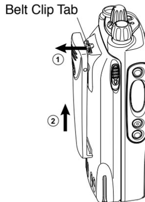
1. Use a key to press the belt clip tab away from the battery.
